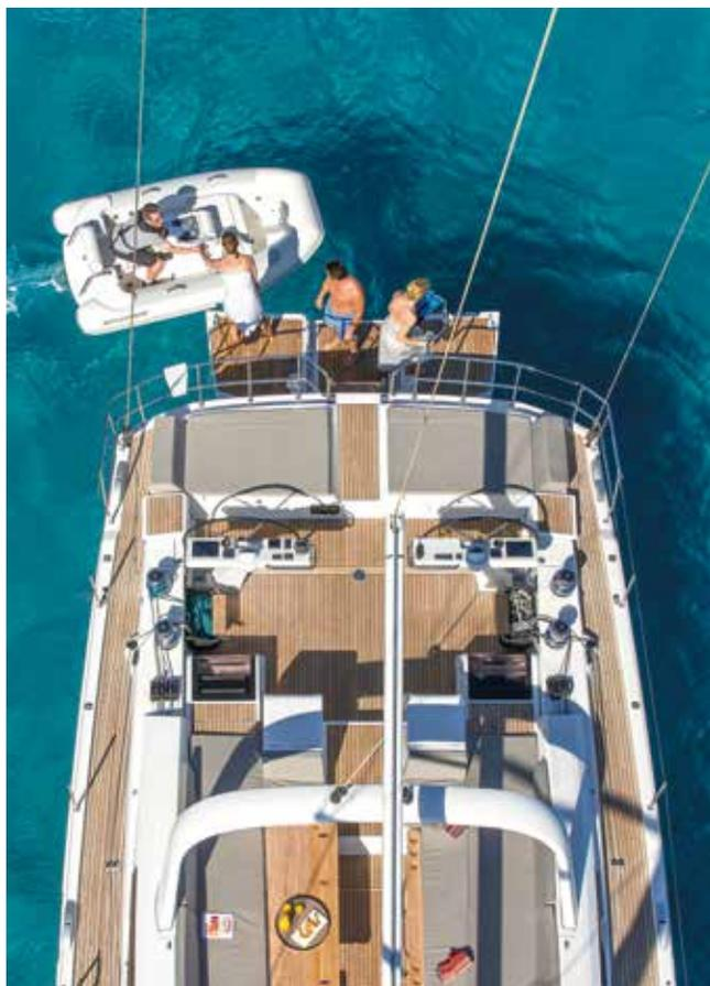
The transom, with a sundeck and a large garage, along with the expansive foredeck, allow for easy handling of different sizes and types of tenders. The traditional transom can be replaced with a flush, walk-through transom for a sportier look and increased floor space in the cockpit.
